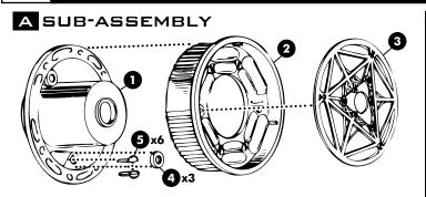
Assemble three pivot pins (5). Once dry, place them in the holes using cement to carefully attach their retainer rings (4). Do not cement pivot pins.
