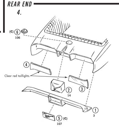
If you are going to paint your car, cement rear roll pan and front roll pan to body and allow time for cement to dry before painting.
