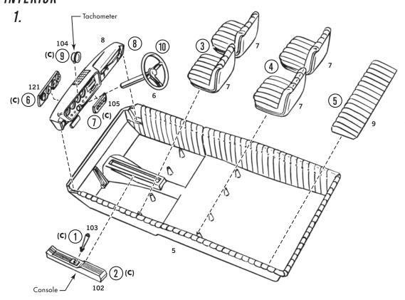
All parts numbered in order of their assembly. Assemble instrument panel before you cement instrument panel to interior.
