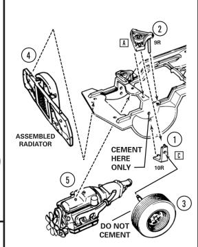
Repeat steps 1 - 3 for other side, using parts 9L, 10L and remaining front wheel assembly.
