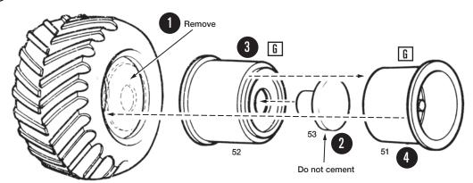
Assemble tires and wheels, two left and two right. Tread should point forward on all four tires.
