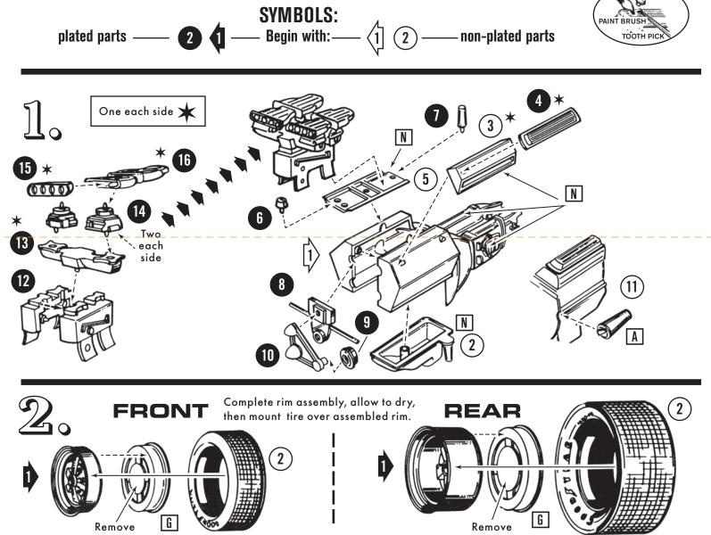
plating from chromed parts where they are to be joined with other parts. Be careful not to get cement on exposed areas. To join parts, use cement sparingly. Apply cement to very small parts with a
