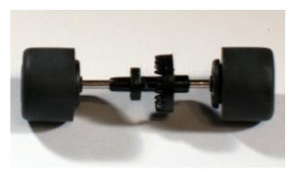
All rims were true and round, no flat spots or odd shapes. The possibility of the rims stripping from the knurls on the axle is a concern. Both rims are flanged on the inside for tire retention/position.
