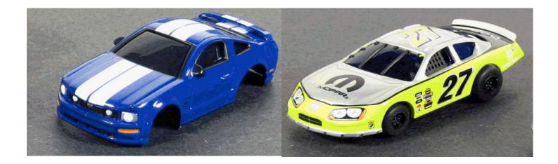
Both cars are cast in a light poly-based plastic. The Mustang weighed in at 6.2 grams (.220 oz.), the Charger also at 6.2 grams . I honestly thought the Charger would come in heavier. Compared to some other cars in my collection these are normal to light in weight.
