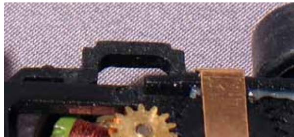
Stock body mount tabs on a pancake chassis (Auto World X-Traction Chassis).
